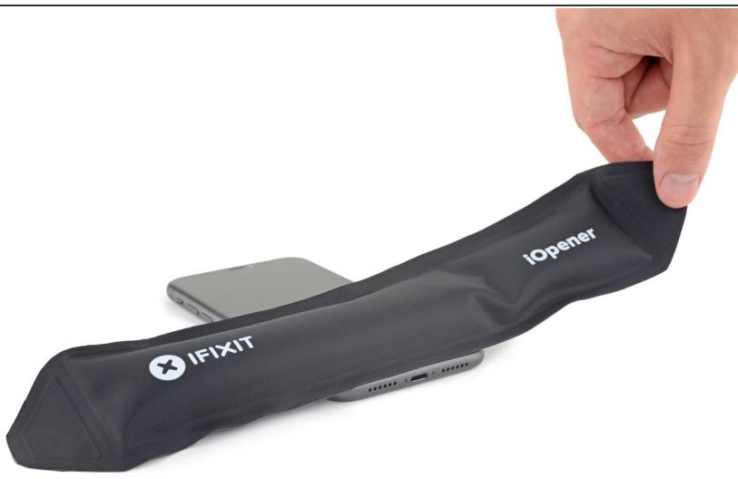
**i** Heating the lower edge of the iPhone helps soften the adhesive securing the display, making it easier to open.
